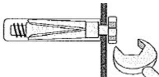
For use with heavier loads such as TV & HiFi Speakers and Satelite Dishes etc.
